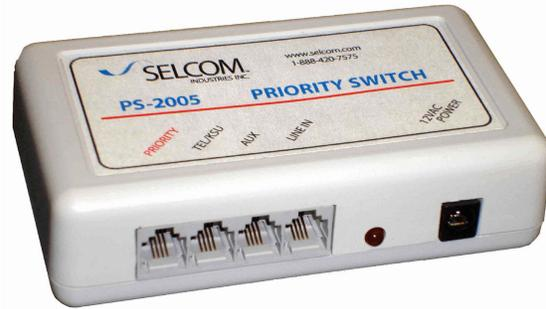
In the idle state, the internal telephone line power supply will be connected to the PRIORITY port & the TEL/KSU port will be connected to the LINE IN jack.
